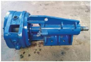
The colloid mill works by shearing, grinding and mixing at high speed. The grinding process occurs by relative motion between particles. It has two teeth, one rotating at high speed and the other fixed, which ensures that the material between the teeth receives a powerful cutting. High frequency vibration and high speed vortex are created. After all; It distributes, emulsifies and breaks the material evenly.
